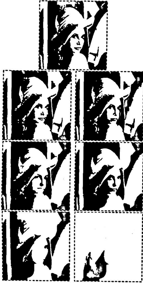
Fig. 3. Bit components of composite images obtained by means of thresholding of Lena's source and segmented images
